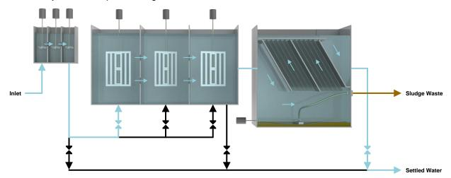
The diagram above shows valve position for three stage rapid mix followed by three stage flocculation and sedimentation.
